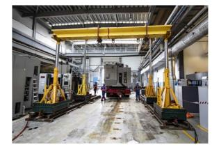
"We'd done all the lift plan and Projector Lifting was just working to our instructions. They supplied the lift gantry while we supplied all the slings and lifting gear. We just lifted the lathe up, got underneath it [with the SPMT], lowered it down and strapped it up. Then we de-rigged the gantry system and moved it down the road, before reassembling it, lifting the lathe onto the skates and pushing it into the shop with a forklift."
